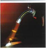
Merit™ LMC6 is a copper coated MIG wire that is an excellent choice for welding on metals with a medium to high presence of mill scale. With its high silicon and manganese deoxidizer levels, superior feedability, excellent arc characteristics, excellent weld appearance and toe wetting, Merit<sup>TM</sup> LMC6 is the industry's premium brand of MIG wires. Shielding gases include argon/carbon dioxide blends and straight carbon dioxide. For best performance use on clean, oil-free base material.
